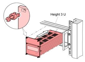
...and fasten the adapter panel to the rack chassis adapter using the screws supplied with the AGC-100.
