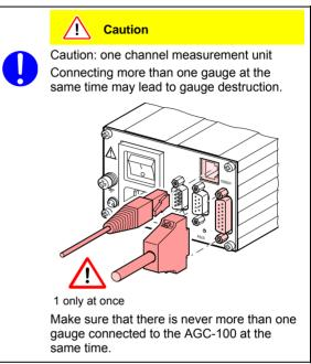
Connect the gauge to one of the two SENSOR connectors on the rear of the unit. Use a screened 1:1 cable (electromagnetic compatibility). Make sure the gauge is compatible ( $\rightarrow \square 9$ ).
