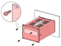
... and secure it with four M3 or equivalent screws.
