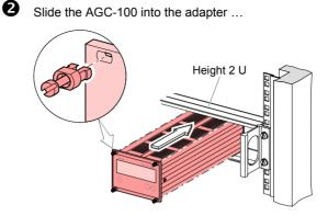
... and fasten the AGC-100 to the rack chassis adapter using the screws supplied with it.
