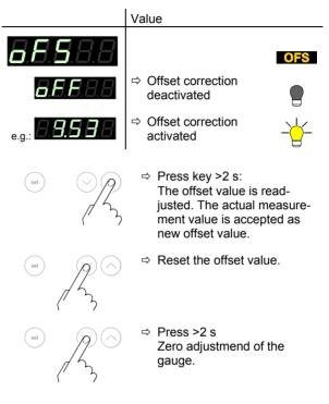
When the offset correction is activated, the stored offset value is subtracted from the actual measurement value. This allows measuring relative to a reference pressure.
