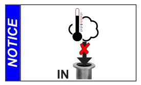
Avoid overheating (e.g., due to hot process gases). Maximum permissible temperature range: see "Gas inlet temperatures", pg. 26.
