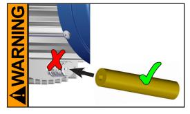
Connect a gas-tight exhaust line at the pump outlet (see above) if necessary. Always vent exhaust gases appropriately (e.g., into a fume hood).
