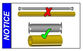
Use connecting hoses with large diameter and keep them as short as possible to avoid flow losses. Locate the pump as closely as possible to the application.
