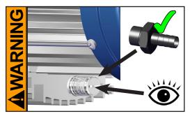
Operation with silencer at the outlet: Operating the pump at a high inlet pressure or pumping dusty gases for a long time may cause clogging of the silencer. Check the silencer regularly and replace if necessary, or install a hose nozzle instead.
