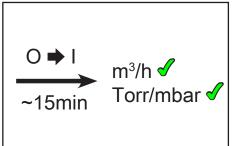
A warm up period (approximately 15 min.) is required to ensure that the rated ultimate vacuum and pumping speed are attained.
