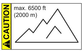
If the pump is installed at an altitude of more than 6500 ft (2000 m) above mean sea level, check compatibility with applicable safety requirements, and adopt suitable measures. There is a risk of the motor overheating due to insufficient cooling.
