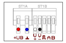
→ Connect the black and the white wire accordingly to the terminal board ST1B (see table above).
