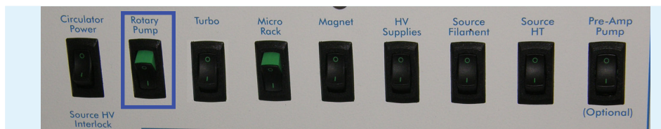
Figure 2.3-5: Switching on the Rotary pump switch.
