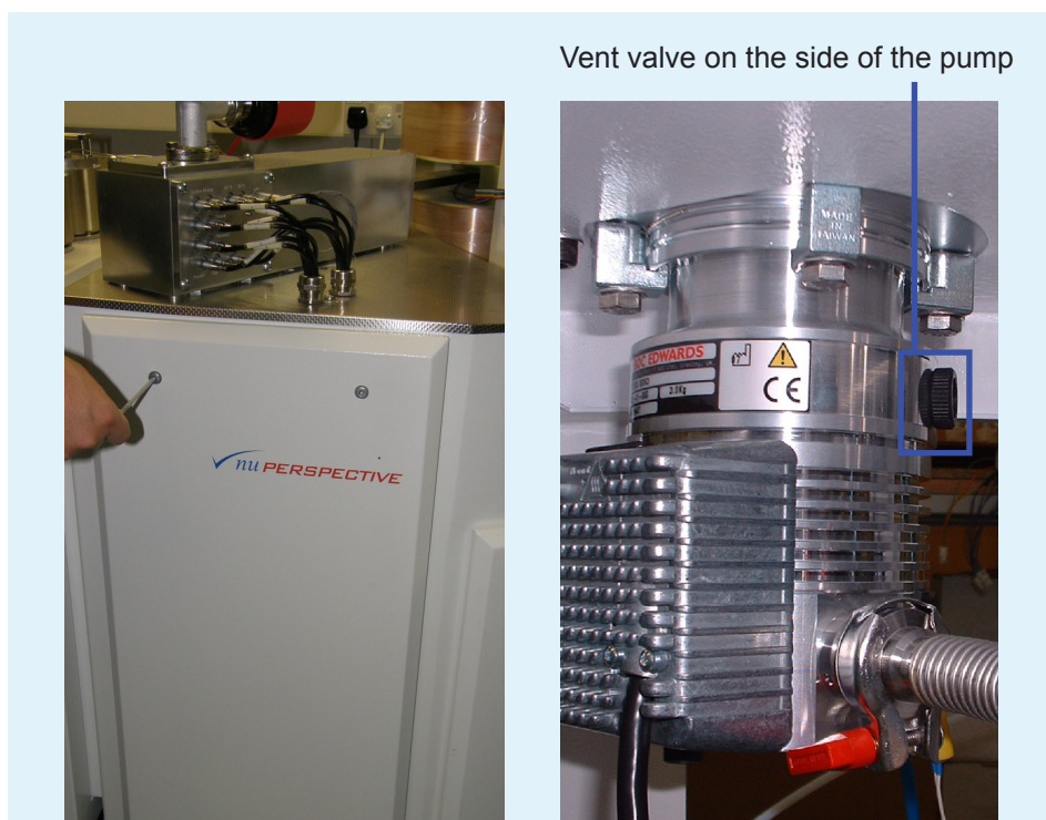
Figure 2.2-5: Removing the panel to open the vent valve on the turbo-molecular pump.
