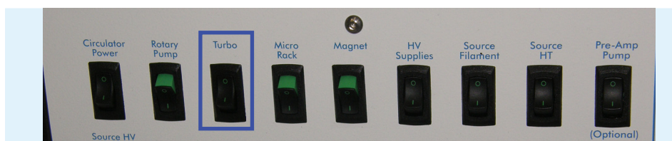
Figure 2.2-2: Switching off the turbo-molecular pumps.
