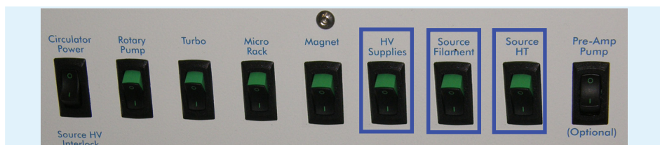
Figure 2.4-5: Switching on the Source Filament, Source HT and HV Supplies.
