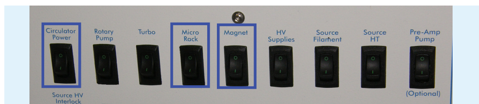
Figure 2.2-6: Switching off the Circulator Power, Magnet and Micro Rack.
