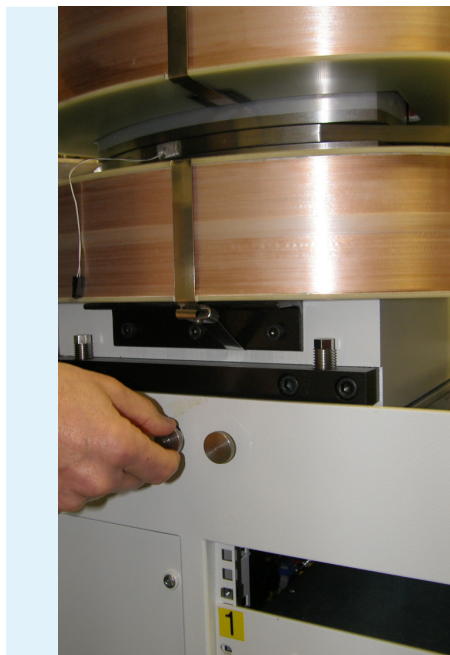
Figure 2.5-15: The locking nut and locating screws on the magnet base.
