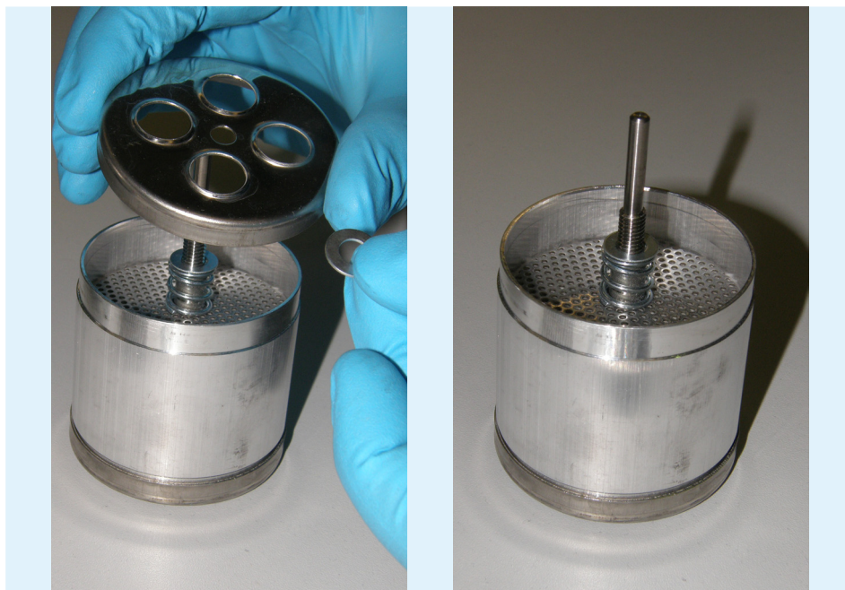
Figure 3.3-7: Removing the end cap, revealing the perforated disc.
