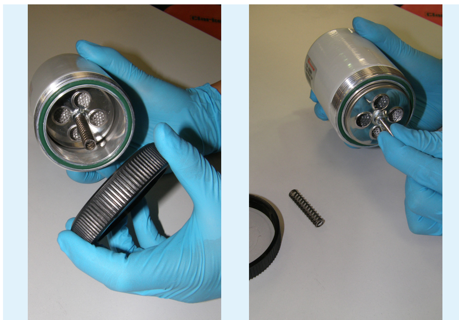
Figure 3.3-5: Opening the foreline trap and removing the spring and cartridge.
