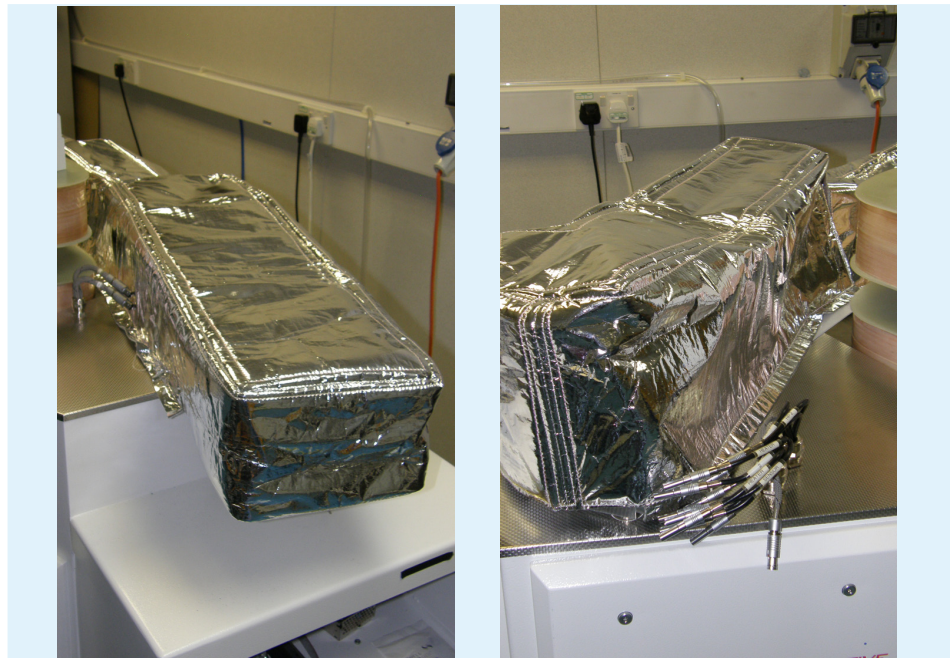
Figure 2.5-18: The bakeout cover fitted over the analyzer housing and the flight tube.
