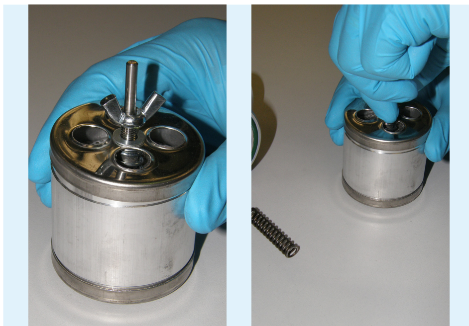
Figure 3.3-6: Opening the cartridge.
