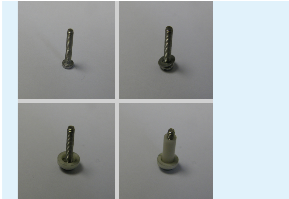
Figure 3.4-36: Building up the repeller screw.
