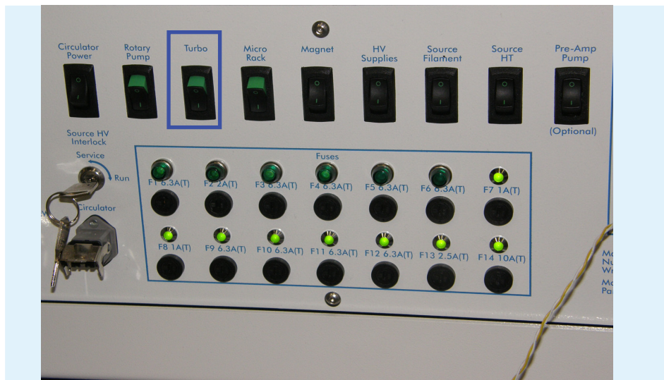
Figure 2.3-6: Switching on the Turbos switch.
