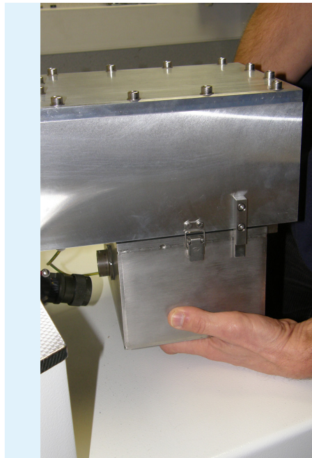
Figure 2.5-7: Checking that the clips of the pre-amplifier housing are secured.
