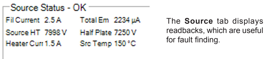
Figure 4.2-1: Source status in the Tuning window.
