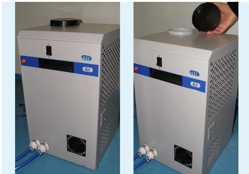
Figure 3.2-2: Checking the water level of the chiller.
