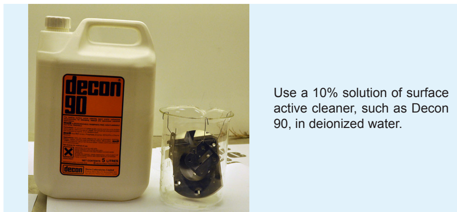
Figure 3.5-2: Placing the stainless steel components in a beaker for cleaning.
