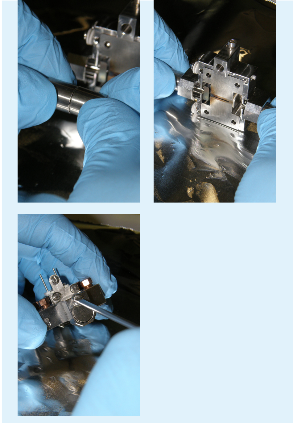
Figure 3.4-54: Placing the magnets back in with the correct orientation.
