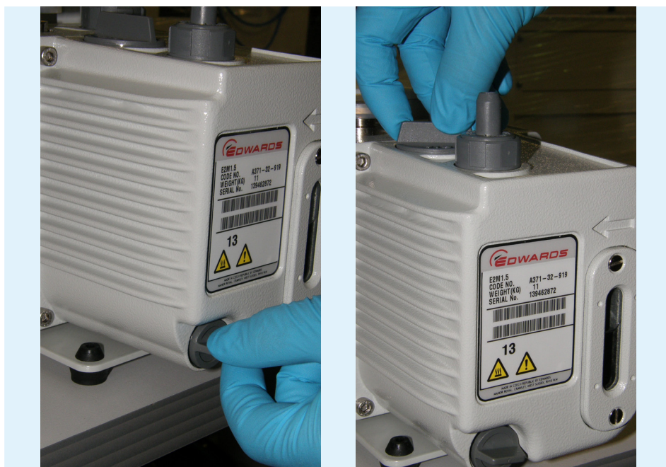
Figure 3.3-3: Removing the oil fill cap and drain plug.
