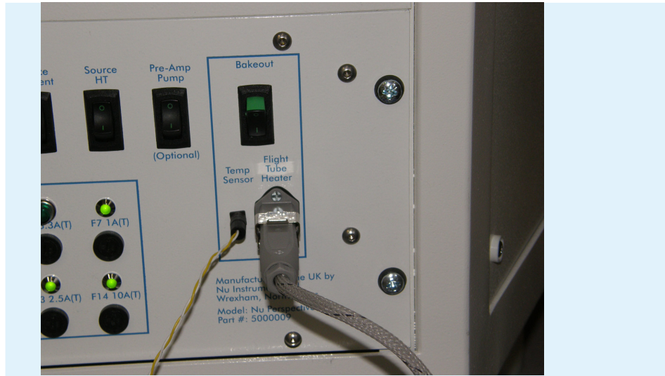
Figure 1.8-4: MDU panel - Bakeout Control.
