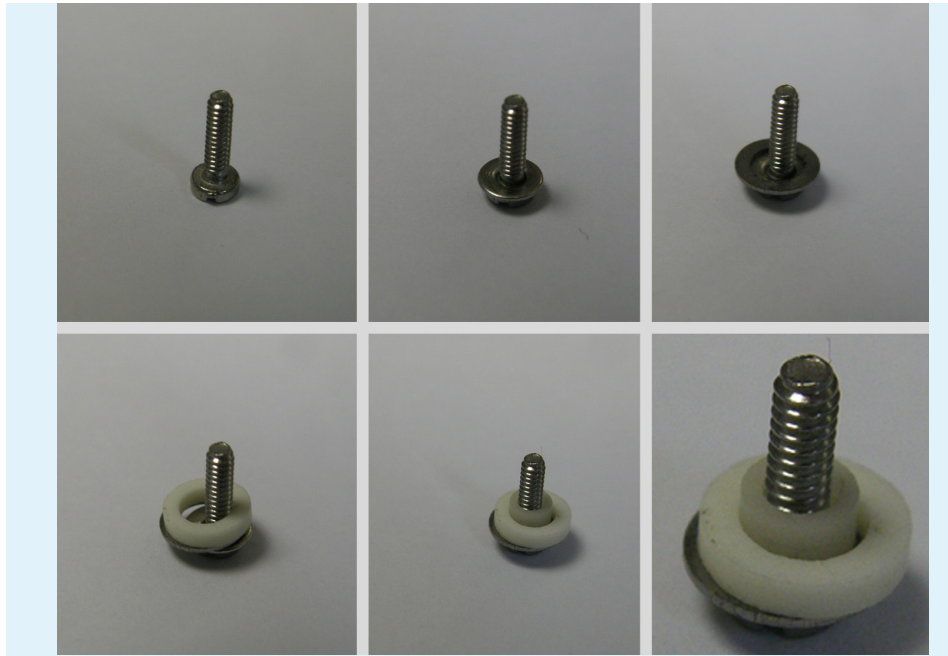
Figure 3.4-45: Building up a trap screw.
