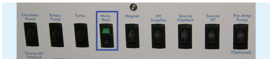
Figure 2.3-1: Switching on the Micro Rack switch.
