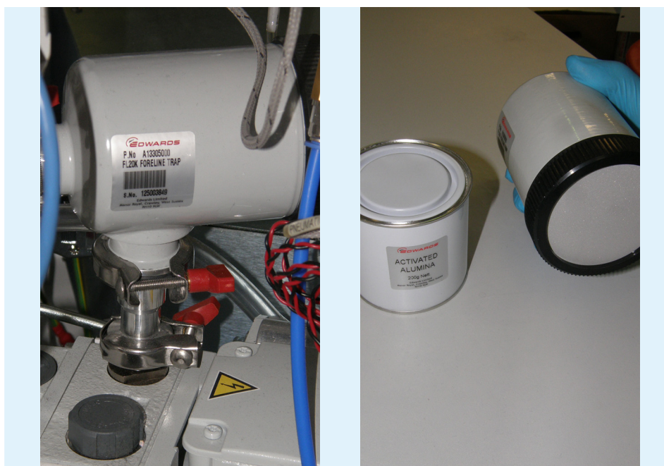
Figure 3.3-4: Removing the foreline trap.
