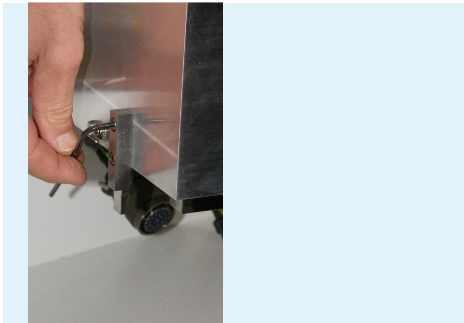
Figure 2.5-12: Re-tightening the bolt.
