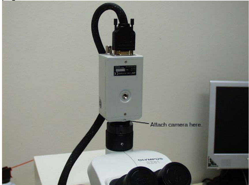
Figure 3-2: Attaching camera after removing from accessory box.
