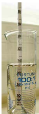
Figure 9-11. Checking density of phosphoric acid
