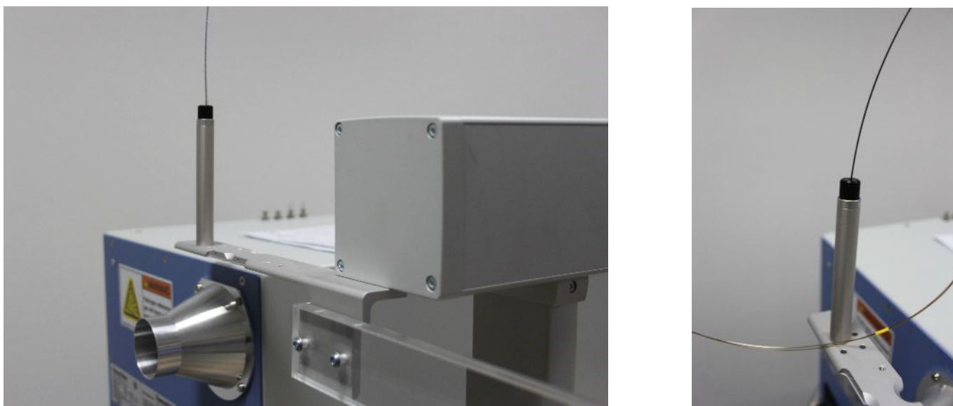
Figure 5-40. Needle line protection jig. The needle line protection wire including connector (BRE0029734) needs to be attached with the connector screw. The needle line protection wire including connector (BRE0029734) is available as spare part.
