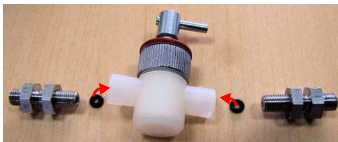
Figure 9-31. Inserting one Viton O-ring into each side of T-piece
