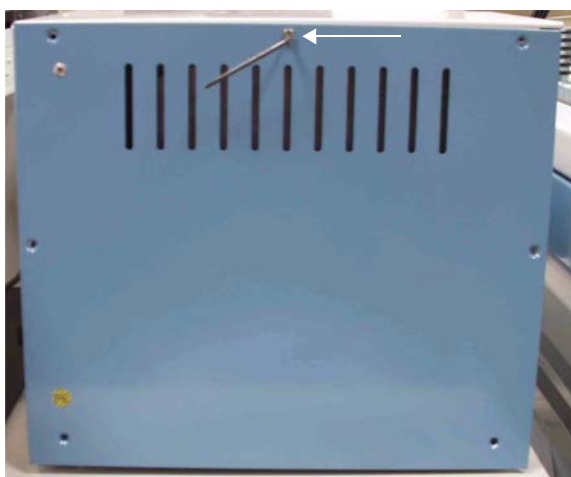
Figure 13-1. GasBench Plus device - opening right side panel
