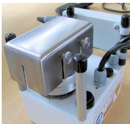
Figure 9-39. Acid pump reassembled
