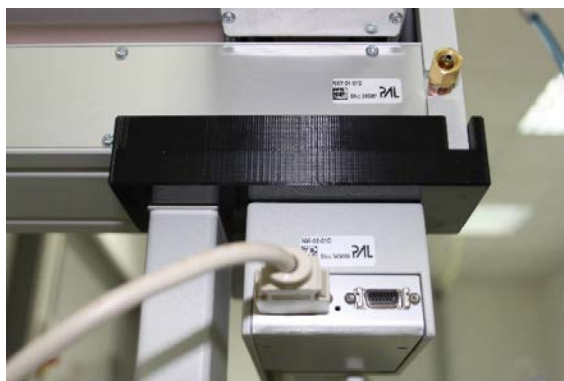
Figure 5-5. Distance calibration tool for TriPlus RSH SMART Std. and Adv.
