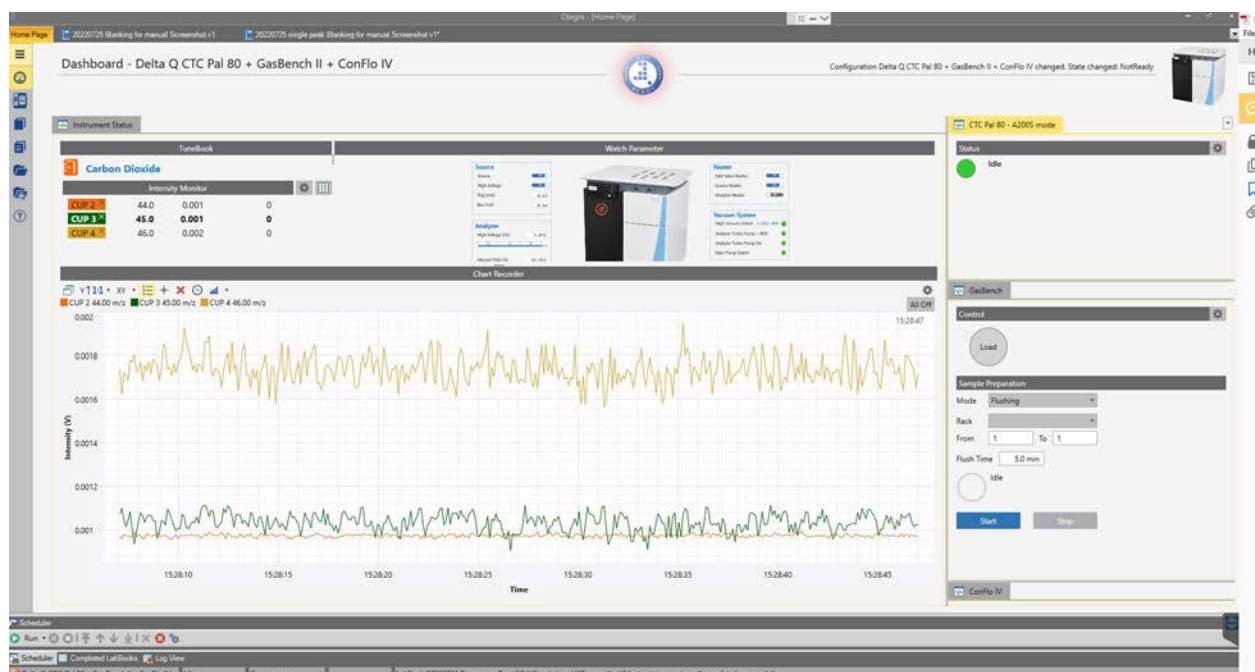
Figure 7-12. Qtegra Dashboard with all peripherals tab. Settings for GasBench II with the CTC Pal 80 autosampler and (as shown here) ConFlo IV
