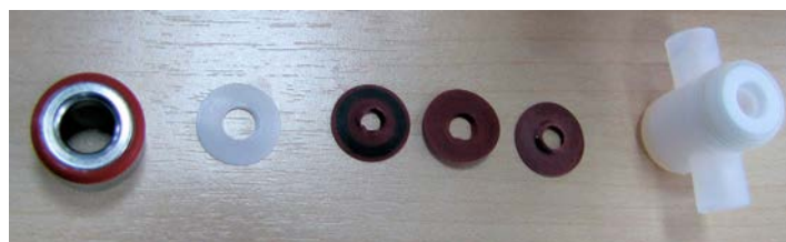
Figure 9-27. Parts resulting from dismantling of acid pump head
