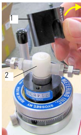
Figure 9-21. Taking away protective cap to access acid pump head
