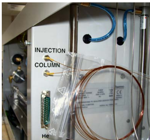
Figure 11-12. PreCon inlet and outlet connections
