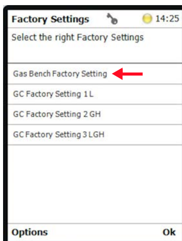
Figure 5-19. Using GasBench Factory Setting for TriPlus RSH for GasBench - Adv
