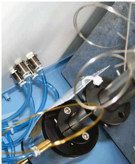
Figure 11-6. Compressed air connections for Cold trap and Dual cold trap
