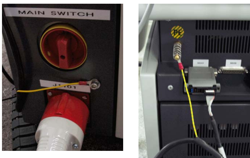
Figure 10. Grounding cable at MAT 253 (left) and DELTA series (right)
