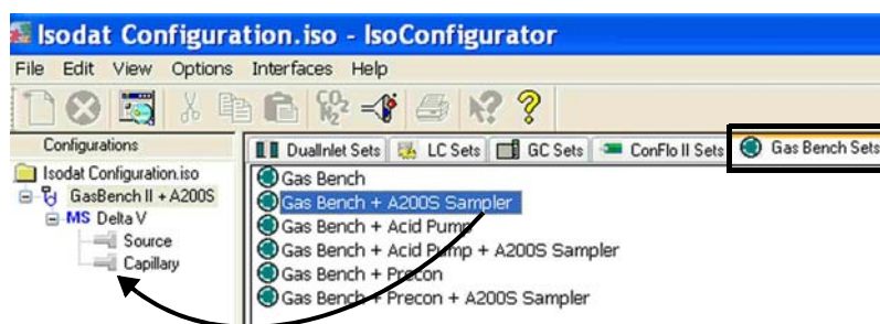
Figure 4-6. Appending GasBench II set to port
