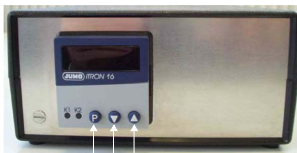
Figure 3-20. JUMO iTRON 16 temperature controller
