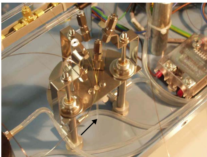
Figure 3-43. Reference inlet (open split)
