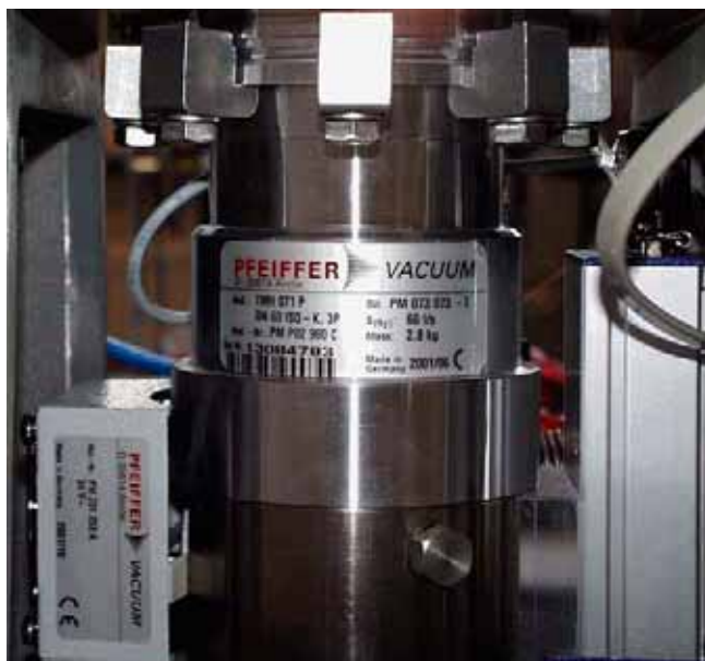
Figure 2-7. Secondary pump (i.e. differential pump)
