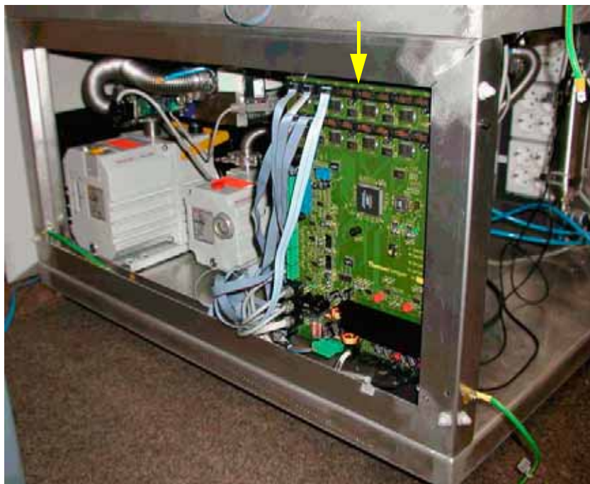
Figure 5-5. Driver board with distributor function
