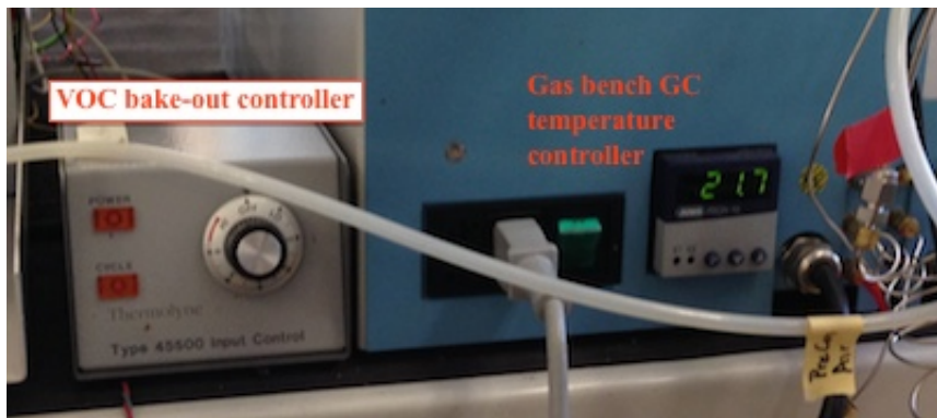
VOC trap temperature controller and GasBench GC controller
