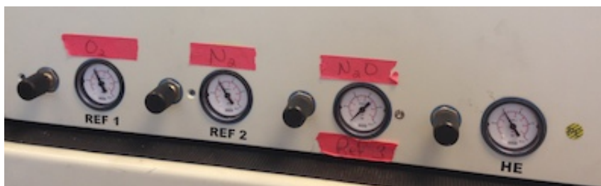
Gasbench pressure gauges
