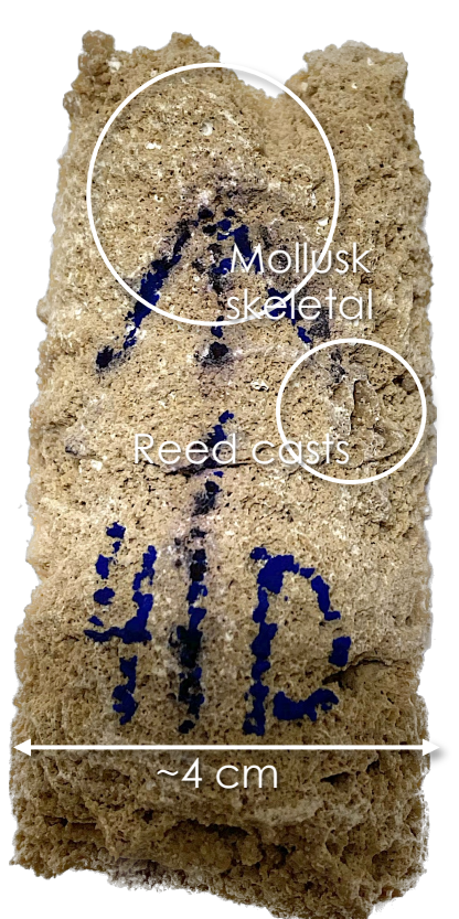
Fig. 2—Travertine sample from Big Thermal Core Hole (location refer to Fig. 4). Organic remains indicate the ambient temperature of the source water.
