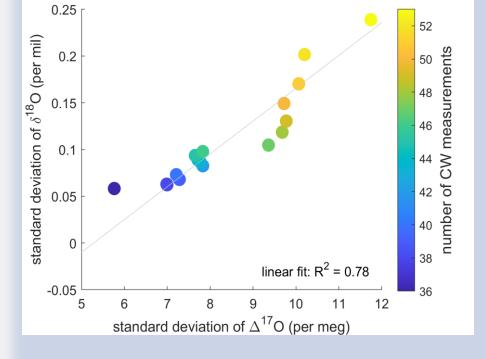
Minimize fractionation of  $\delta^{18}$ O, since it is associated with error in  $\Delta^{17}$ O.
