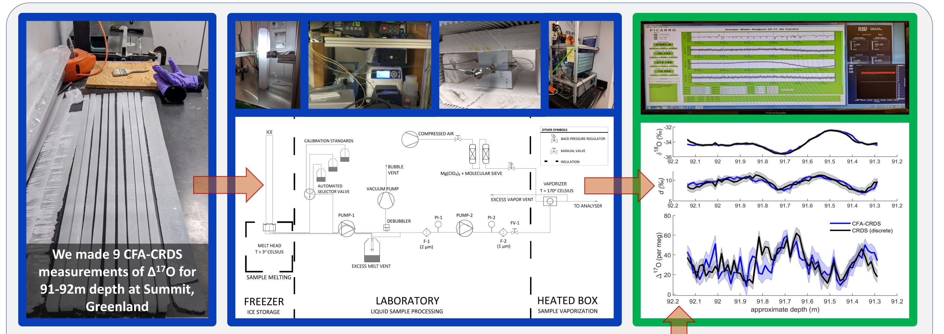
We designed a continuous-flow analysis (CFA) system to measure water isotopes ( $\delta^{17}O$ ,  $\delta^{18}O$ ,  $\delta D$ , d, and  $\Delta^{17}O$ ) by cavity ring-down laser spectroscopy (CRDS). We measure replicate ice-core sections with this system to study the reproducibility of  $\Delta^{17}O$  by CFA-CRDS and to examine the remaining sources of uncertainty in the measurement.  $\Delta^{17}O$  from ice cores should provide new information about earth's climate history.
