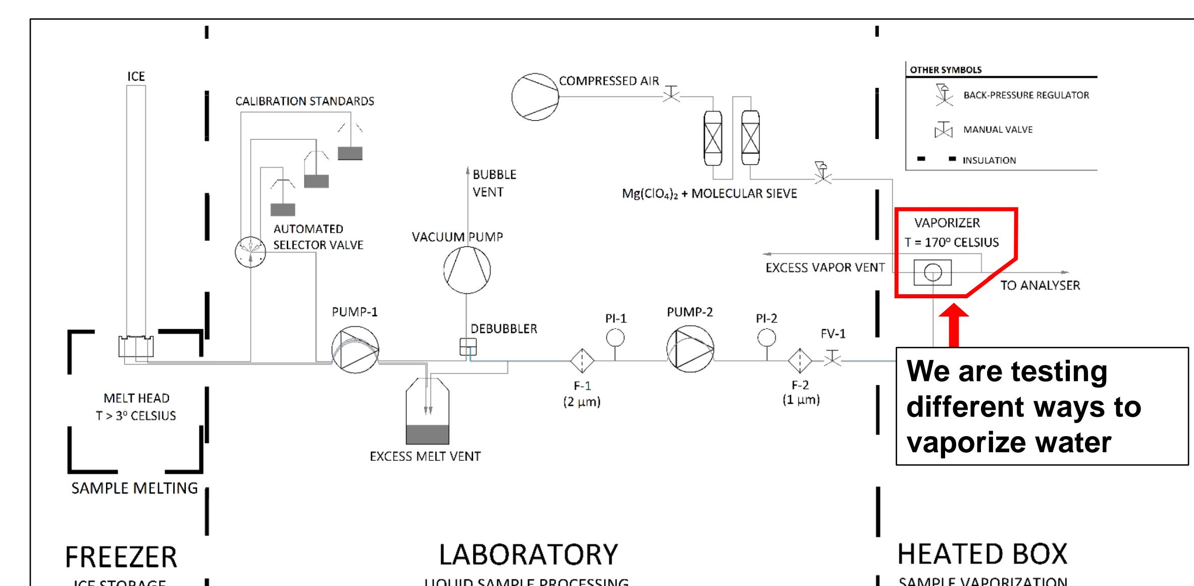
Figure 1: Process flow diagram for our CFA system. Thick dashed lines indicate transitions between temperature-controlled process spaces. Note that F-1 and F-2 are filters, PI-1 and PI-2 are pressure sensors, and FV-1 is a flow valve.
