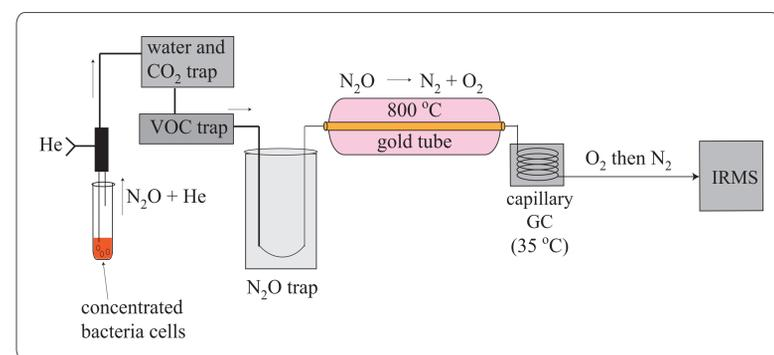
Figure 4 - Plumbing diagram of the nitrous oxide pyrolysis system.  $\text{N}_2\text{O}$  generated from nitrate via bacterial denitrification is purged from head space vials, purified, cryofocused and then passed through a gold tube held at 800 °C. Pyrolysis products,  $\text{O}_2$  and  $\text{N}_2$ , are separated in a capillary GC and then into an isotope ratio mass spectrometer for 32, 33, 34 and then 28, 29 mass / charge measurement (adapted from Kaiser et al., 2007).
